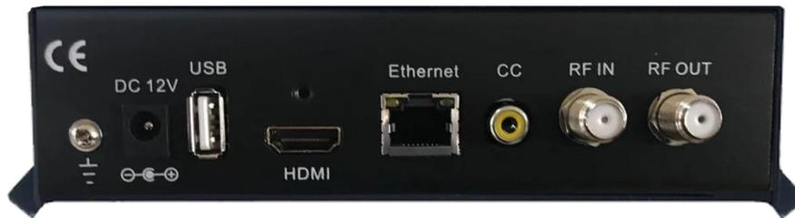
**Grounding:** to connect the earth cable
